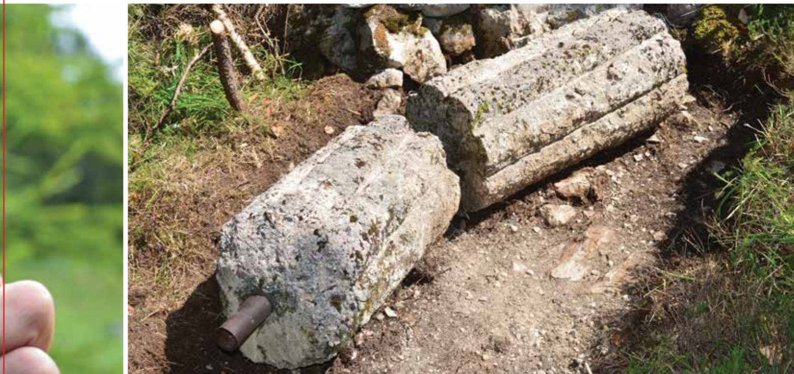
Za graditelji ceste je med drugimi ostal tudi betonski valjar, ki so mu po opustitvi odstranili kovinska prečna rebra, katerih odtisi se poznajo v betonu (foto: Uroš Košir, 2022). Inter alia, a concrete roller used by the road builders remained, with the metal cross ribs removed after it had been abandoned. Their imprints are still identifiable in the concrete (photo: Uroš Košir, 2022).
